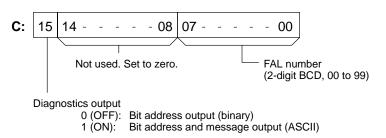
Logic Diagnostic Instructions If the time until the logic diagnostics condition goes ON exceeds T, the logic diagnostic instructions are searched for the OFF input condition. If more than one input condition is OFF, the input condition on the highest instruction line and nearest the left bus bar is selected.
